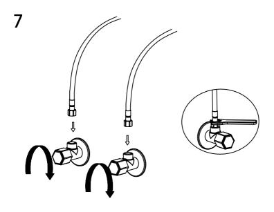
7. Connect the hot & cold supply lines onto the matching water valves and secure the connection with an adjustable wrench.
