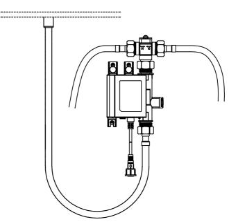
6. Cold water pipe connect to mixer valve inlet(mark C). Hot water pipe connect to mixer valve inlet(mark H).
