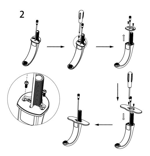
2. For 3-hole sink.use the screwdriver to remove the base at the bottom of the faucet.replace with the deck plate.and secure the deck plate to the bottom of the faucet.
