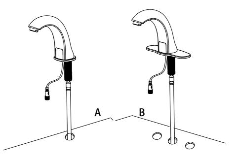
**1.A.**For 1-hole sink.insert the cable flexible pipe and the stem into the bottom of the faucet into the sink' s mounting hole.then attach the faucet on the sink.
