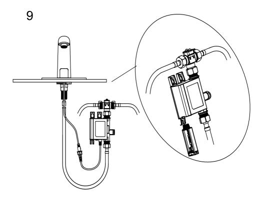
9. Remove the battery pack cover and take out the battery pack; insert 2 AAA batteries. put the battery pack back in the control box and replace the cover firmly.
