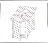
7. Turn the cylinder valve on the tank clockwise to close the propane tank. Attach the preassembled regulator from the body to the cylinder valve by turning the regulator coupling nut clockwise. Make sure it is fastened securely and tighten connections by hand only.
