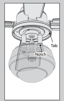
Lift the globe and align the notches in the globe with the tabs in the light kit. Attach the glass bowl to the light kit by twisting it clockwise until it snaps into place.
