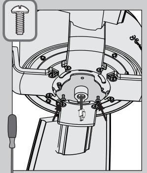
Screw two housing assembly screws from
