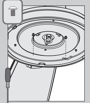
Screw two housing assembly screws from
