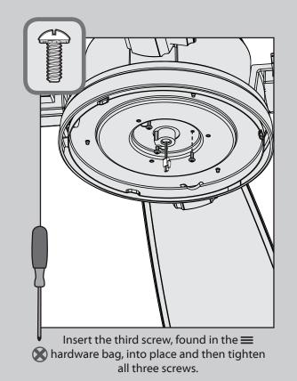
Make sure the upper switch housing is securely attached to the mounting plate. Failure to properly secure all 3 assembly screws could result in the switch housing fixture falling. Light Kit
