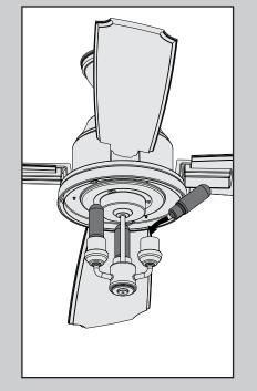
Install a bulb into each of the sockets. When necessary, replace with bulbs of the same type and wattage.
