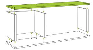
Start with the bottom horizontal zBoard (there will be holes on only one side of board). Align vertical zBoards to holes in the horizontal zBoard.
