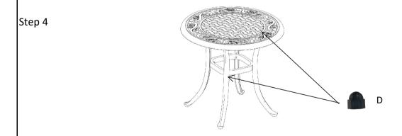
Tighten all Nuts with Wrench. And Turn over the table. Adjust the pre-installed Rubber Pad (L) until the Table is level with the ground ,Tighten all the nuts and cover them with nut caps(D). Your table can use now.
