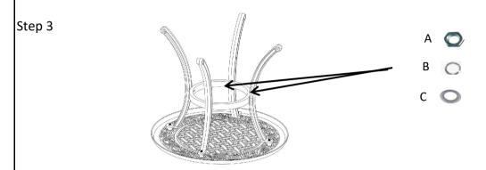
Attach the Table legs Support (3) to the four Legs (2) using flat washer, spring washer and nuts (A,B,C)DO NOT over tighten.
