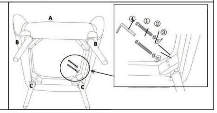
Insert the Back Leg(B) into the mounting position of Chair (A).
