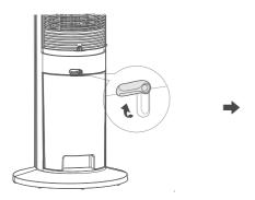
3 Unscrew the rotary knob in "—" shape manually (90 anticlockwise) to separate the water tank from the water pump module (including the water pipe).
