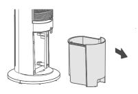
6 After feeding water or cleaning the water tank, install the water pump module in the water tank. Insert front hook into the slot of the water tank, and then rotate rotary knob in "—" shape clockwise for 90, and close it as shown in the figure.
