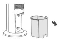
4 Pull out the tank completely to clean and add water.
