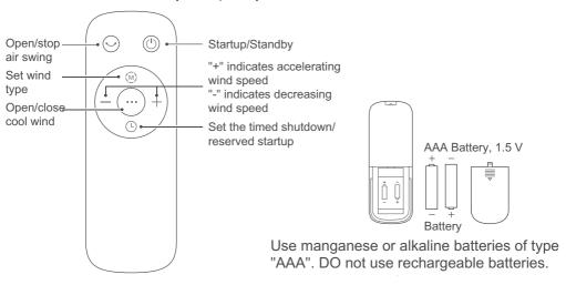
Note: Both machine body operation " ( are buttons of cool wind are buttons of cool wind
