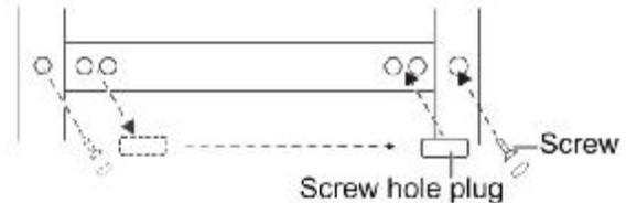
14. Install the center hinge to the left side with the two screws you removed previously.
