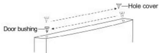
13. Remove screws and the center hinge screw hole plug on the left side of the cabinet, then install in the screw holes on the right side of the cabinet.
