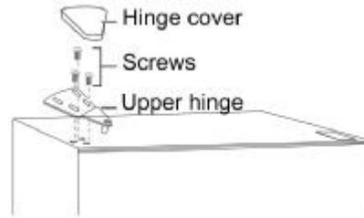
19. Secure the upper hinge to the top left side of the cabinet with the three screws you removed previously. Before you tighten the upper hinge screws, make sure that the top of the door is level with the cabinet and that the rubber gasket makes a good seal.
