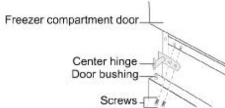
15. Remove the screw that secures the door stops from the bottom right of the freezer compartment door, then remove the door stops and install to the bottom left side.
