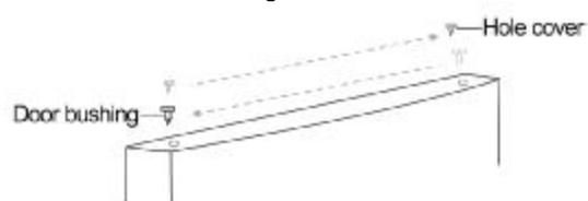
18. Remove the screw that secures the hinge screw hole cover from the top left side of the cabinet, remove the cover and secure the cover on the top right side of the cabinet.
