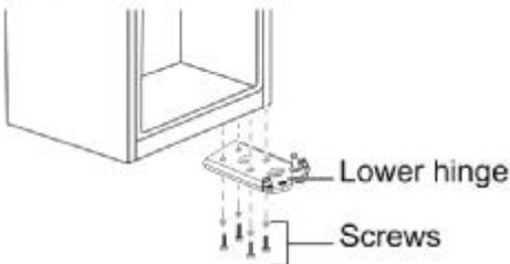
7. Remove the washer and nut that secure the pin shaft to the right hole on the lower hinge, then remove the shaft and pin screw.
