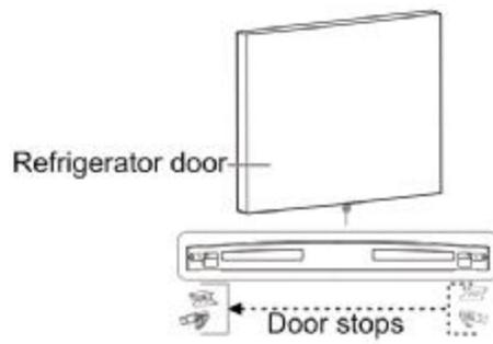
11. Install the refrigerator compartment door.
