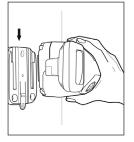
7. Line up the light with the mounting plate and slide the light into the grooves.
