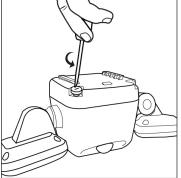
2. Use a screwdriver to loosen the four screws on the back plate. The screws will not come out all the way.
