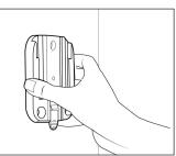
6. Determine mounting location for the light. Place the mounting plate on the surface so that the tab is pointing down and mark the pilot holes for drywall. Use a drill to insert the anchors, then line up the mounting plate with the holes and drill screws in.
