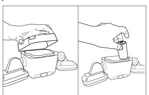
3. Lift the battery lid off the back of the light. Insert 4 D-Cell batteries with the flat ends against the springs.
