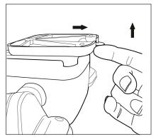
1. To remove the back plate from the light, use your finger to push up on the mounting bracket tab. This will unlock the bracket. Then slide the bracket down off the back of the light.
