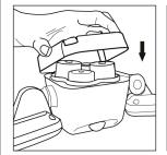
4. Replace the battery lid and make sure the screws are twisted in tightly.
