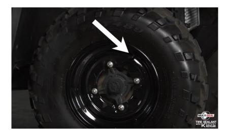
1. Ensure the tire has been rotated where the valve stem is near the top of the tire (between 10 and 2 O'clock degrees)
