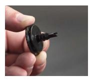
5. Gently tug and twist to remove the disc from the tube. The disc is your valve core remover tool.
