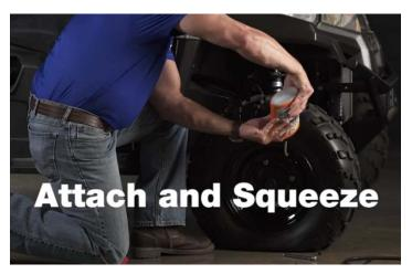
9. After allowing the tire to deflate, push the bottle sealant tube onto the open valve stem, thereby connecting the bottle and tube to the valve stem. Once you have ensured a good connection, hold the bottle upside down, and gradually squeeze the bottle until the recommended amount of sealant has gone into the tire.
