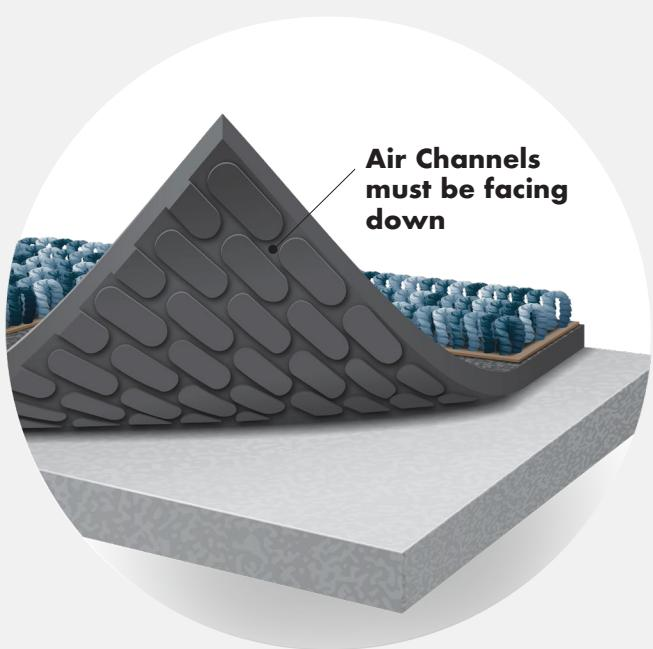
For stretch-in carpet, cushion shall be installed up to the edge of the tack strips and be securely fastened to the subfloor using staples or tape at the seams and 25mm to 150mm (1" to 6") within the perimeter edges all around the installation to prevent shifting.
