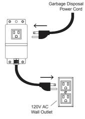
Plug the garbage disposal into the air switch control box. Plug the air switch control box into the wall outlet.
