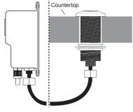
Push the ends of the air tubing through the small plastic nuts. Firmly press one end of the air tubing into the Air Switch, and the other into the Air switch control box.
