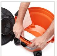
Push cardboard collar onto inlet and behind rib(s) so that cardboard is flush against inside of drum.
