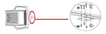
Attach the Iron Plate to the Seat.
