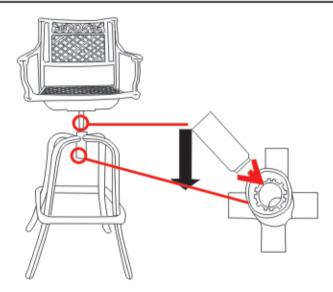
Attach the Seat with attached Iron Plate to the Chair Leg Base as pictured above.
