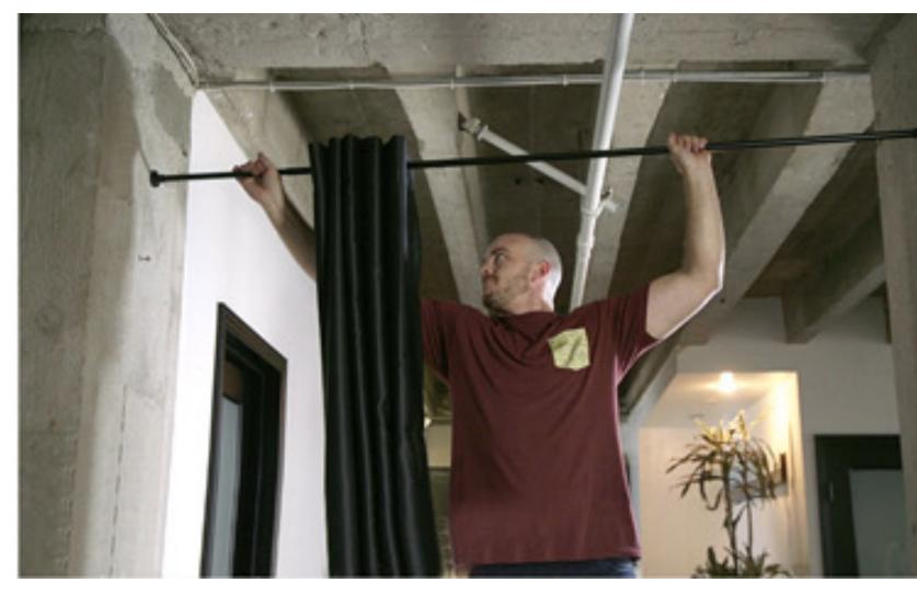
8. Place one end of the rod at the desired position on the opposite wall. Push the rod against the opposite wall with enough force to cause the rod to reduce in size. You can then bring the end closest to you up to it's final position and release.
