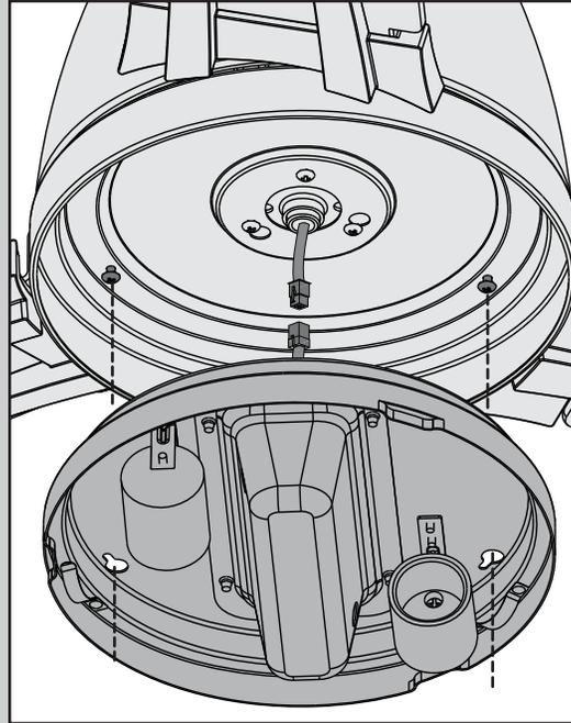
Connect the plugs from the upper and lower switch housings. Make sure to line up the colored markings on the connectors. Wrap light kit keyhole slots around the screws and twist counterclockwise.
