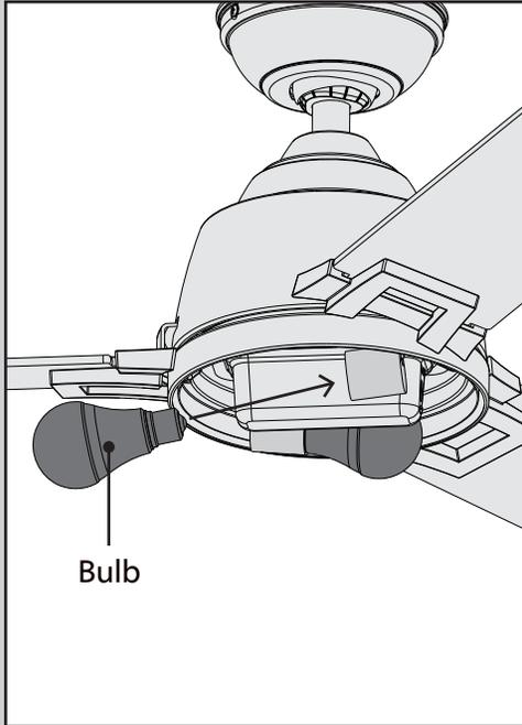
Install a light bulb in each socket.
