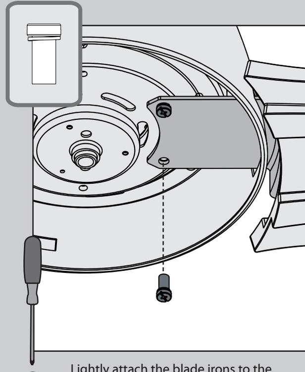
⊗ Lightly attach the blade irons to the motor with screws found in the ☒ hardware bag, then securely tighten after both screws are attached. Repeat this step for each blade assembly.
