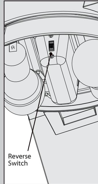
To switch the direction of air flow, move the reverse switch to the opposite position. You will need to remove the glass to do so.
