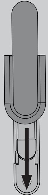
Slide the cradle onto the mounted bracket.
