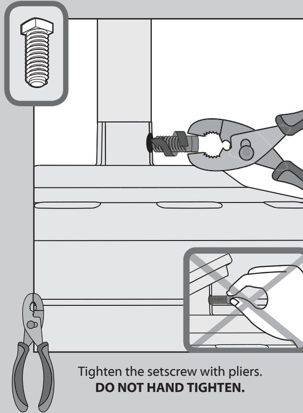
Tighten the setscrew with pliers.
