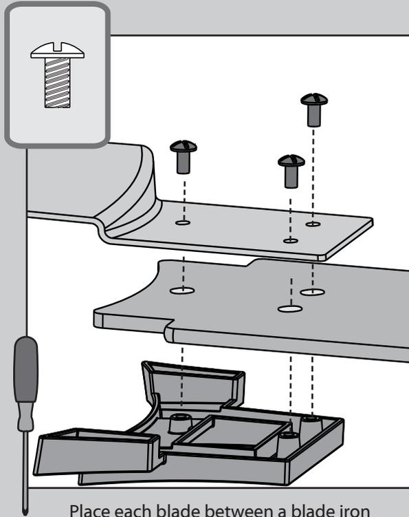
⊗ Place each blade between a blade iron and medallion. Install three blade screws, found in the ▲ hardware bag, to attach the medallion to the blade iron. Repeat this step for each blade.
