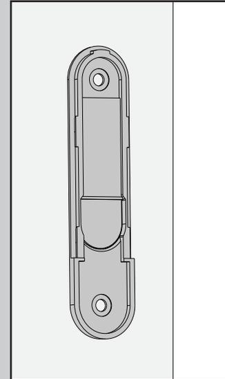
Press the cradle bracket against the wall and hold firmly for 30 seconds.
