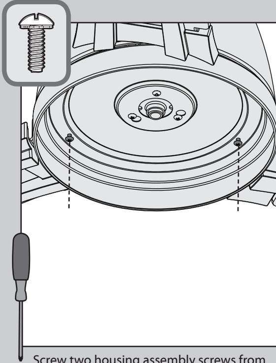
⊗ Screw two housing assembly screws from the ≡ hardware bag halfway into the upper switch housing.
