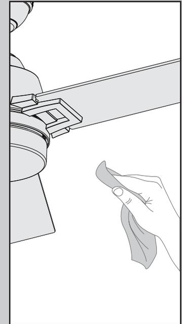
**Cleaning the fan** - use soft brushes or cloths to prevent scratching. Cleaning products may damage the finishes.
