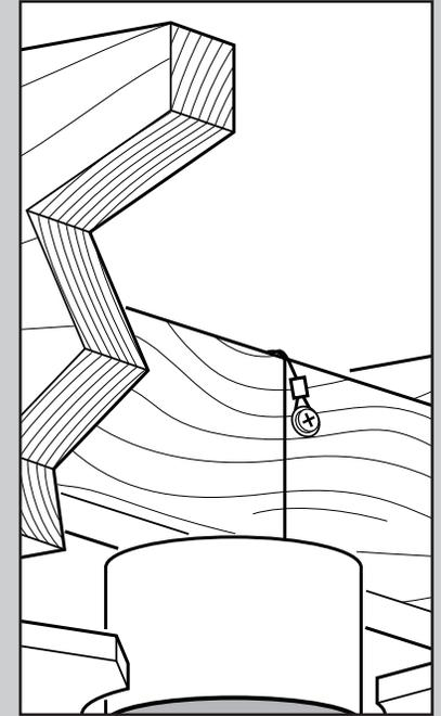
Insert the looped end of the braided cable through the ceiling bracket and one of the holes in the outlet box into the ceiling. Access the support brace in the ceiling. You may not be able to do this from below the ceiling depending on your installation site.
