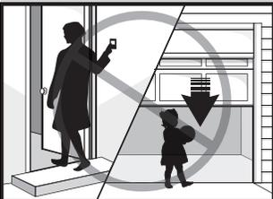
**Keep the door in sight until it completely closes** when using the wall-mounted push button or transmitter.
