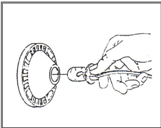
**CAUTION:** The replacement bulb must be the same rating as the factory installed bulb.
