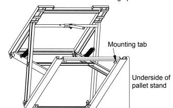
2. When you receive the caster kit, the caster clamping brackets (2) will still be attached to the caster bracket weldment (1). Use a pair of pliers to bend the mounting brackets back and forth until they snap off of the weldments.
