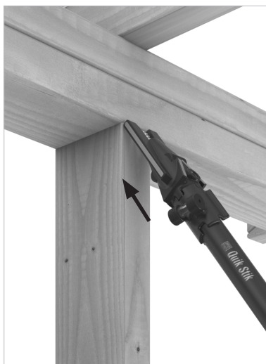
Installation 4: Rafter/Truss Aligned with Stud or Over a Window/Door Header: Fasten from Narrow Face of Stud.
