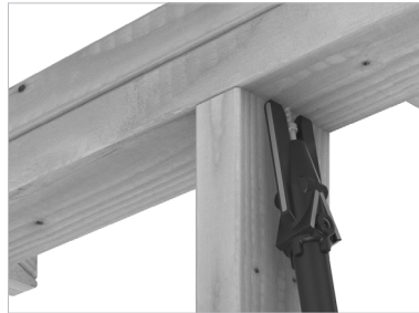
Retracting the Quik Stik head allows screw point and threads to be visible.
