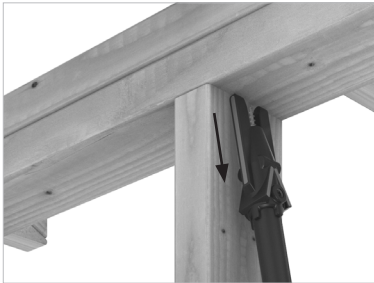
Retracting the Quik Stik head allows screw point and threads to be visible.
