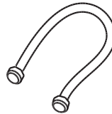
Toilet water supply line
