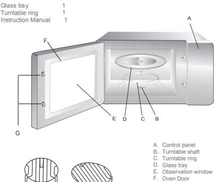
Grill Rack (Only be used in Convection function and be placed on the glass tray)
