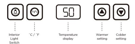
Please note that the actual interior cabinet temperature in a thermal electric unit is dependent on the ambient (room) temperature. You may set the cabinet temperature within the operational range but due to high ambient temperature the unit may not reach the selected temperature.
