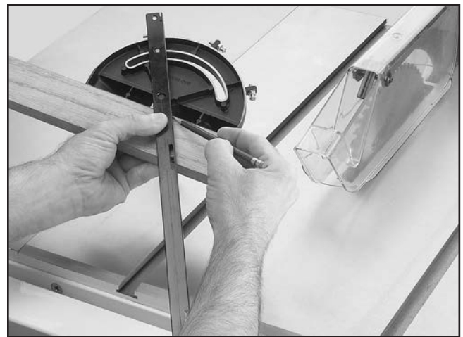
Figure 43. Example of marking miter line.
