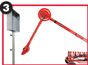
Align with conduit, properly adjust booms
