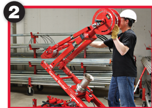
Flip booms into position and lock
