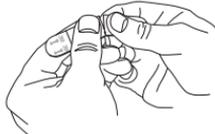
3. Remove the red liner. Press the adhesive strip onto one of the top corners of the back of the antenna. Repeat for the other top corner. Then place a single mounting strip on the metal section in the bottom middle of the antenna, with the strip facing down.
