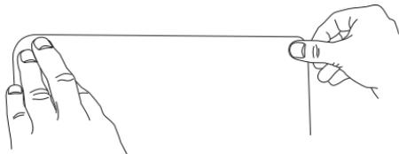
6. Stop pressing the antenna against the wall and confirm that it's firmly attached to the wall. Then press an additional 30 seconds.
