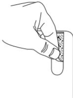
5. Line up the antenna where you want to put it, then press it against the wall for 10 seconds.
