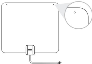
**To mount the antenna using thumbtacks (not included):**
