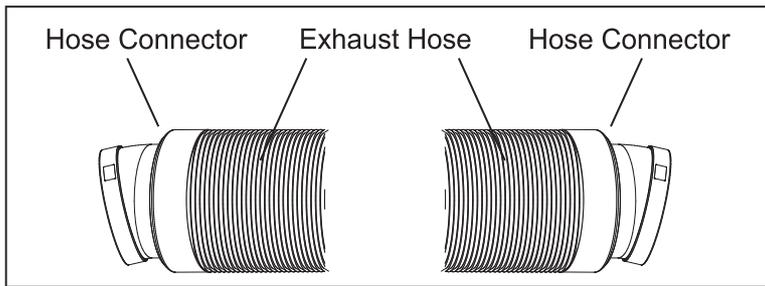
3. Align the tab cut-outs of each of the hose connectors to the tabs on the air exhaust and air intake at the rear of the unit and snap in place.
