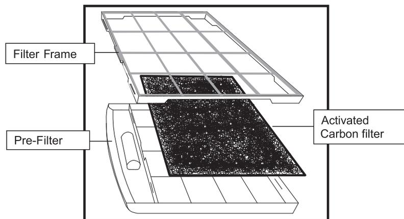
An optional 3M™ Filter can also be purchased to replace the activated carbon filter. The 3M™ Filter has an agent that helps inhibit the growth of mold and mildew on the filter. This filter is electro-statically charged for enhanced particle capture and retention.
