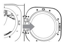
Move the door to the left side and line up the holes in the hinge with the holes in the cabinet.
