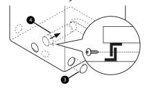
Preassemble a 4" (10.2 cm) elbow 6 to the next 4" (10.2 cm) duct section, and secure all joints with duct tape. Be sure that the male end of the elbow faces AWAY from the dryer. Insert the elbow/duct assembly through the side opening and press it onto the adapter duct. Secure it in place with duct tape. Be sure that the male end of the duct protrudes 1.5" (3.8 cm) to connect the remaining ductwork. Attach the cover plate 6 to the back of the dryer with the included screw.
