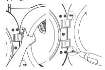
**9** Insert the latch on the right side and install the latch screws.
