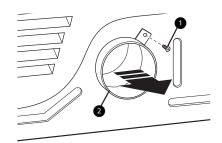
Press the tabs on the knockout and carefully remove the knockout for the desired vent opening. (Right-side venting is not available on gas models.) Press the adapter duct onto the blower housing and secure to the base of the dryer as shown.
