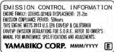
An **Emission Control Label** is located on the engine. (This is an EXAMPLE ONLY, information on label varies by engine FAMILY).
