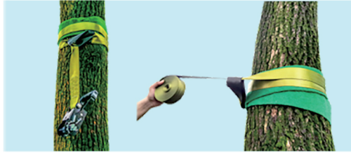
2. Noose the ratchet end and long line around 2 suitable trees or anchor points min 1 circumference.
