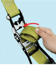
5. Feed line through the bolt on ratchet. Pull through all the slack, until the line is tight.
