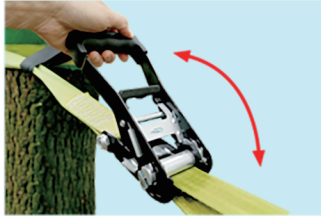
6. Pull the handle up and down to tighten up the ninja line.
