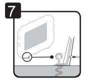
Stand the Airblown® Inflatable Movie Screen<sup>TM</sup> upright, ensuring that fans are located on the bottom. Locate the 8 Base Stakes and screw them into the ground through the provided holes in each leg of the stands.
