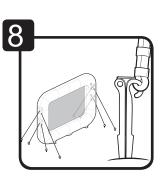
Insert the 8 tether stakes into ground and attach clips from nylon tethers to tether stakes, as shown.
