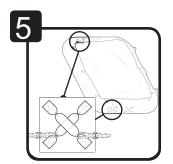
Attach 2 long nylon tethers to the upper "X"-shaped nylon strap on each side of the Airblown® Inflatable Movie Screen $^{TM}$ .
