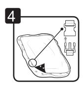
Attach Movie Screen<sup>™</sup> to frame by connecting the clips along the edges and corners of the Movie Screen<sup>™</sup>. Locate the four legs on the bottom of the frame and unfold them completely.
