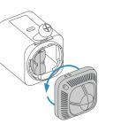
Then, remove the battery and discard the orange battery insulator.
