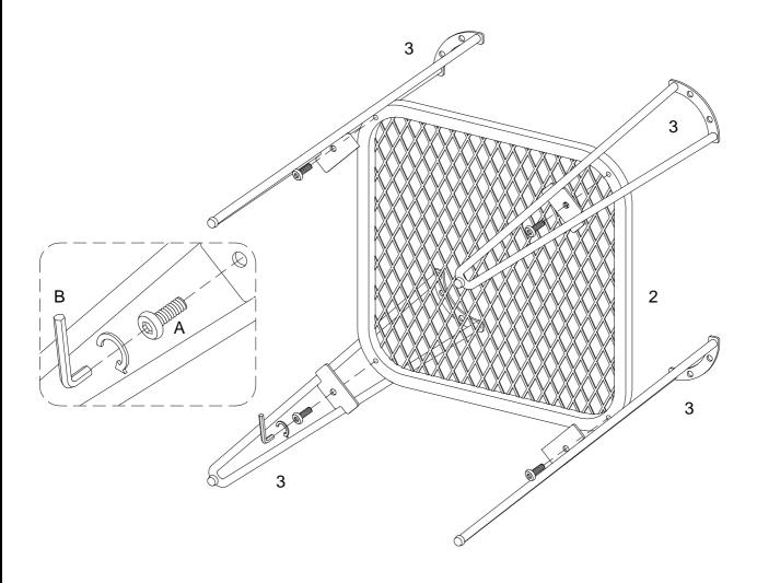
Attach part (2) to part (3) using bolt (A) with hex key (B).
