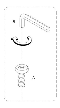
Attach part (3) to part (1) using bolt (A) with hex key (B).
