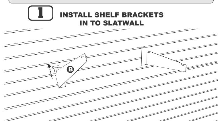
Insert Brackets (B) in to grooves in slatwall from 22" to 26" apart.
