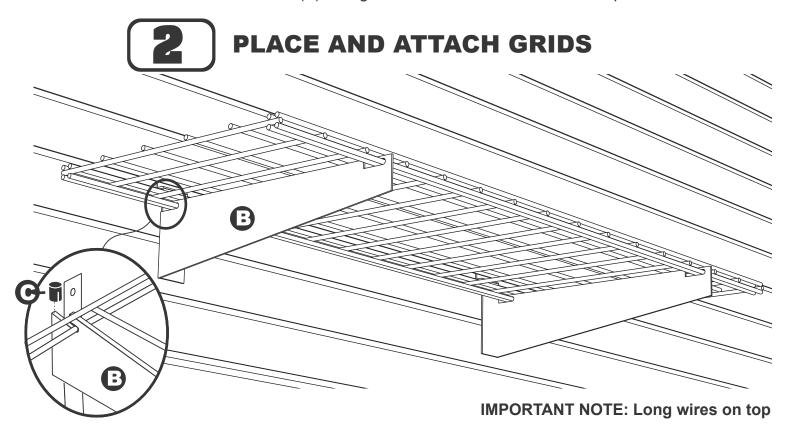
Place Grids (A) on top of Brackets (B) and into slots with long wires on top. Pull shelf forward to lock in place.
