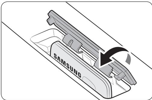
4. Insert the upper area of the adapter cover first, and then press to lock as shown.
