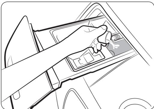
Add only liquid chlorine bleach to the **bleach compartment**. Do not exceed the **max line**.
