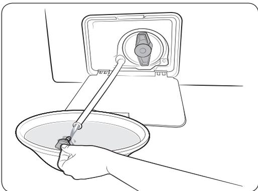
4. Open the tube cap and let water in the **Emergency drain tube (B)** flow into the container.
