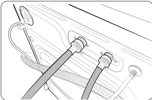
5. Connect the other ends of the water hoses to the corresponding inlets on the rear of the machine as specified. Make sure the hot water hose is connected to the hot inlet, and the cold water hose to the cold inlet.
