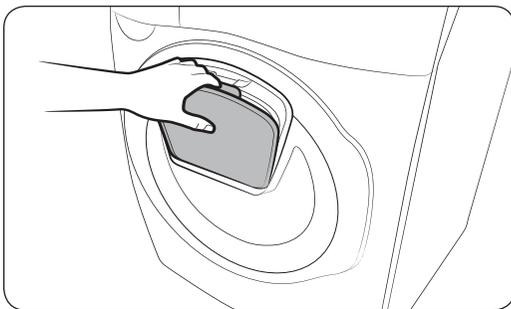
3. Open the Add Door and insert additional laundry into the drum.
