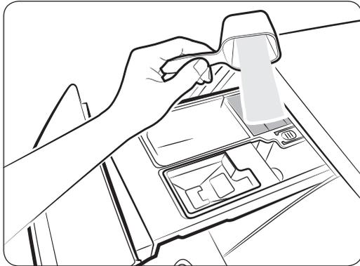
3. Add fabric softener to the **softener compartment**. Do not exceed the **max line (A)**.
