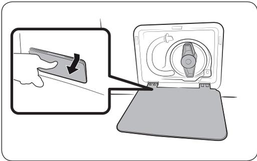
1. Power off the washer, and then unplug it from the electrical outlet.
