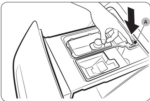
1. While holding down the **release lever (A)** inside the drawer, slide open the drawer, and then remove the drawer from the washer.
