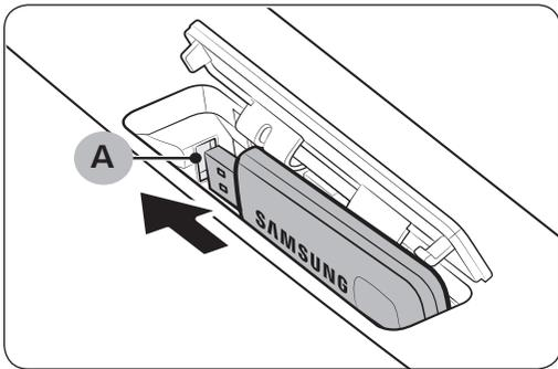
3. Insert the SmartHome Adapter into the **Adapter port (A)** in the correct direction. Make sure the Samsung logo faces forward.
