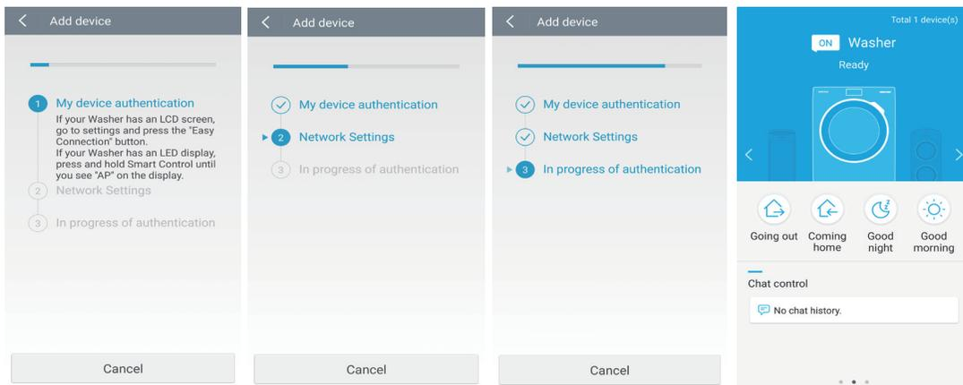
6. Press and hold **Smart Control** on the washer for more than 5 seconds until the “**AP**” message appears on the display. Your washing machine is registered with the app.
