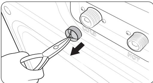
4. Use pliers to pull out the mesh filter from the inlet valve.
