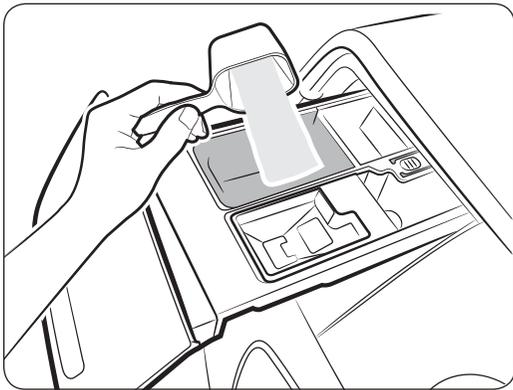
First, remove the provided liquid detergent container from the main-wash compartment. Then, add powdered detergent to the main-wash compartment according to the detergent manufacturer's instructions.
