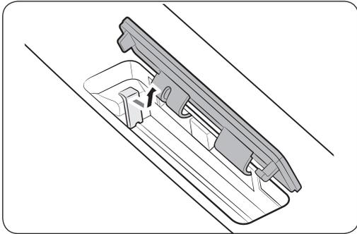
2. Open the adapter cover to reveal the protective cap of the adapter. Gently pull the cap to the right and lift up to remove.
