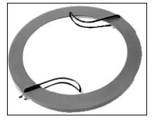
Use blade protectors to protect blade teeth during unit transportation.
