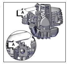
clockwise to increase idle speed; counterclockwise to decrease idle speed.
