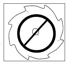
When sharpening a blade, always remove the same amount of materials from each tooth to maintain balance. A blade that is not balanced will cause unsafe handling due to vibration and can result in blade failure.
