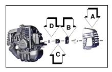
Note: When cleaning carbon deposit, be careful not to damage the catalytic element inside muffler.
