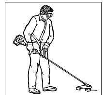
During blade operation, the same fatigue reduction is achieved. Safety to the operator is also enhanced by reducing the possibility of blade contact with the operator's hands and feet by restricting trimmer movement.
