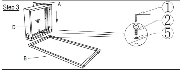
Attach Left Leg(B) to Backrest(A) and Seat Panel(D) using Bolts(②) and Washers(⑤) with Allen Key(①).
