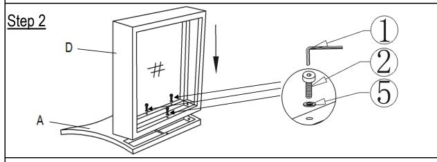
Attach Seat Panel(D) to Backrest(A) using Bolts(②) and Washers(⑤) with Allen Key(①). **Do not fully tighten the Bolts.**
