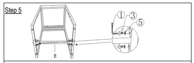
Attach Footrest (E) between the Legs using Bolts(3) and Washers(5) with Allen Key(1). **Do not fully tighten the Bolts.**
