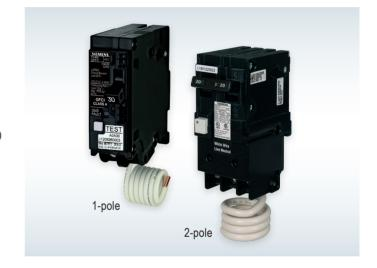
Siemens GFCI circuit breakers are UL Listed and CSA Certified as Class A devices. Current imbalances of 4-6 milliamps or more between load conductors will cause the ground fault sensor to trip the circuit breaker.
