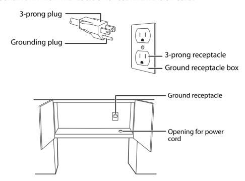
If the power supply cord is too short, have a qualified electrician or serviceman install an outlet near the appliance.
