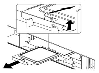
6 Remove the LED module and replace only with an equivalent 1.2 watt LED bulb.
