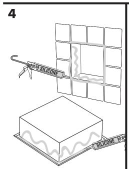
Generously apply silicone on all sides, on the inner surface of the edge of the niche, on the wall and on the uprights (as illustrated) for optimal sealing and support.
