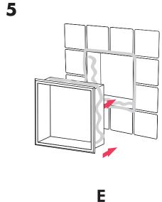
Place the niche against the wall and press firmly. Remove the niche and add silicone if it does not protrude slightly.
