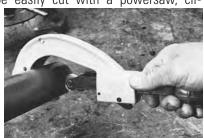
suitable for circular saws; band saw speed should be approximately 3,000 ft./min. Carbide-tipped blades are preferable when quantities of pipe/tube are to be cut. To insure square-end cuts, a mitre box, hold-down, or jig should be used. Pipe or tubing cutters can be used for smaller diameter pipe/tube when the cutting wheel is specifically designed for plastic pipe.
