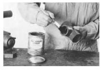
3. Put a second full even layer on the pipe/tube O.D.
