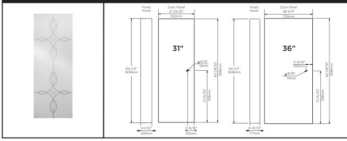
MATERIALS: 1/4" (6mm) Tempered Glass Panel (Large panel). 3/16" (4.16mm) Tempered Glass Panel (Fixed In-Line Panel).
