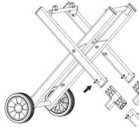
• Secure Cart Leg Assembly, Bottom Leg Connector and Bottom Leg Assembly with 16 Screws (Part N) as shown.
