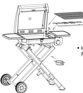
• Install Flame Tamer (Part B), Grill Grate (Part C) and Drip Tray (Part D) as shown.
