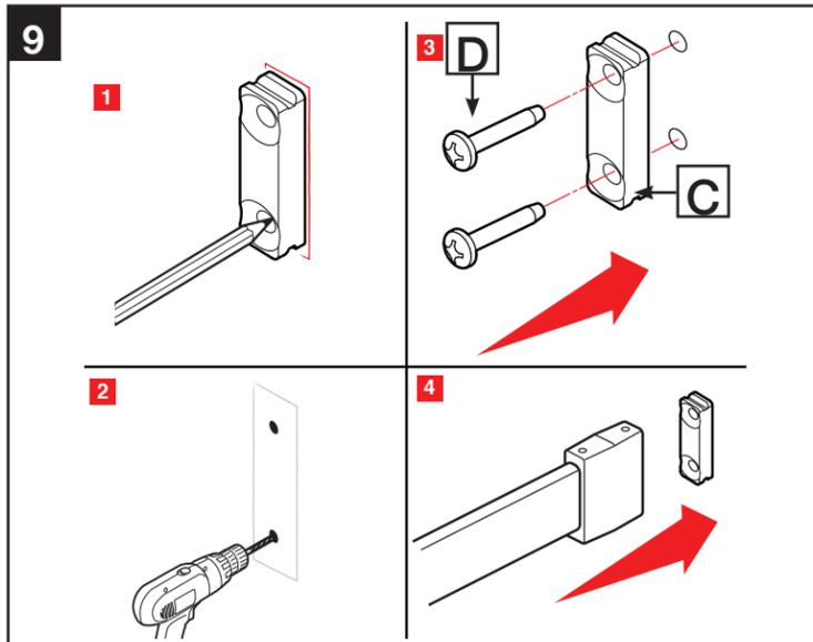
Mark holes for the bracket. Drill holes through wall material using a 3/16" drill bit (for tile walls, use a glass and tile bit). Then use a 9/64" drill bit to drill holes into studs. Install wall bracket [C] using (2) M4 x 38mm screws [D]. NOTICE: Screws must go into studs.
