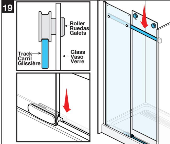
Hang the glass on the track. Make sure the glass goes into the inside slot on the guide block and the rollers seat on the track. CAUTION: Door installation requires two people.
