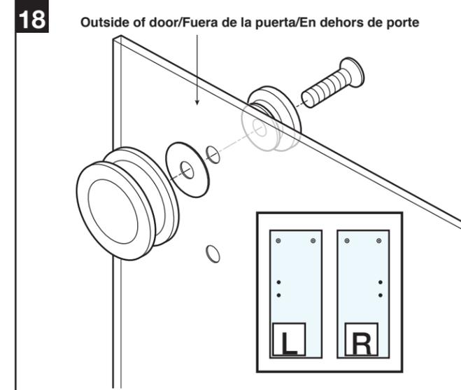
Install rollers. Do not tighten completely until after any height adjustments have been made.
