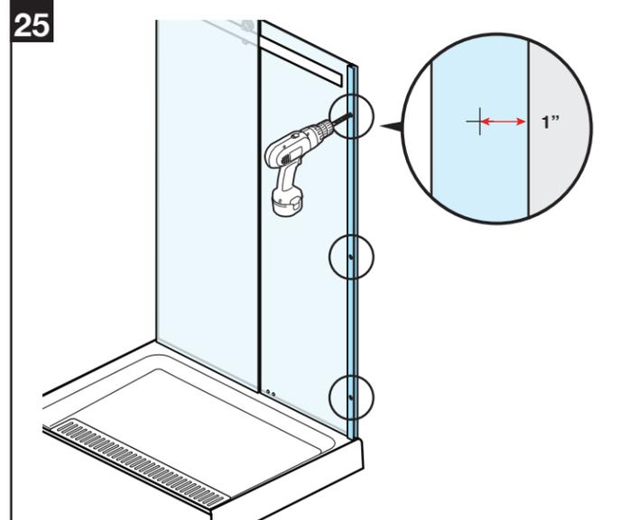
From inside the shower, drill three pilot holes into the glass panel frame and wall jamb using 1/8" drill bit. Holes should be 1" from the wall and evenly spaced on the top, middle, and bottom of the frame.
