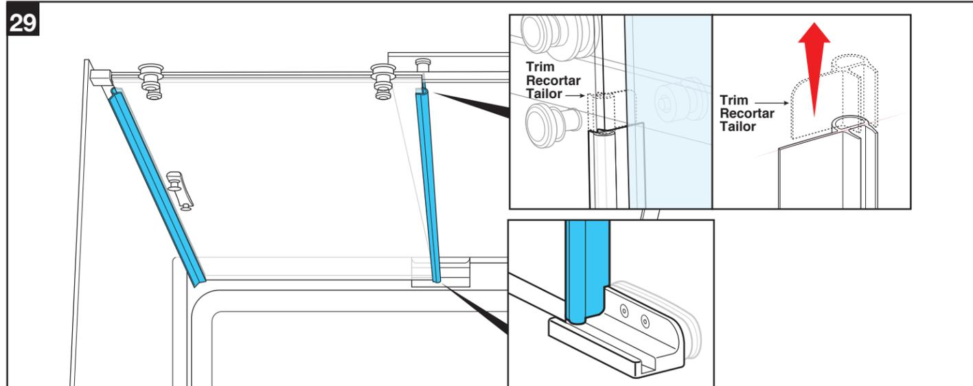
Install door gaskets. Trim inner gasket as shown.
