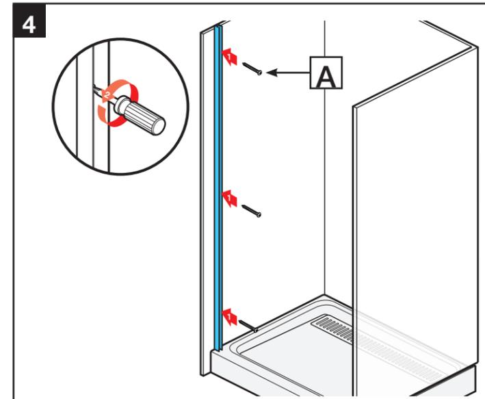
NOTICE: Screws must go into studs. Install wall jamb using (3) M4 x 38mm screws [A].
