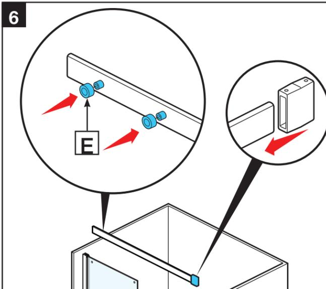
Slide spacers [E] onto the track bosses. Slide wall mount bracket onto the end of the track.
