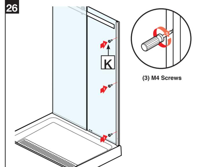
Secure the glass panel frames to the wall jambs using (3) M4 screws [K].
