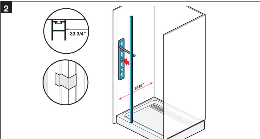
Measure 33-3/4" from the finished back wall and mark a line. Using a level and wall jamb, extend a plumb line up the wall. Position the wall jamb so that the inside edge is even with the marked line. Hold it in place with tape. Check that the wall jamb is plumb.
