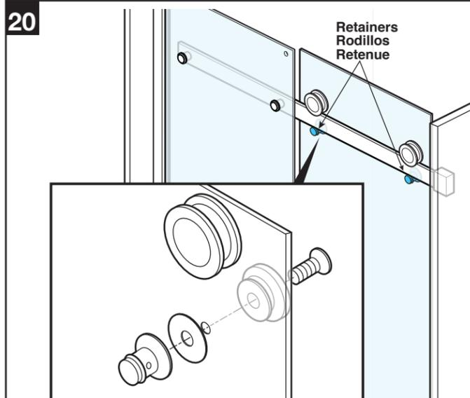
Install door retainers [H]. Do not tighten completely until after any height adjustments have been made.
