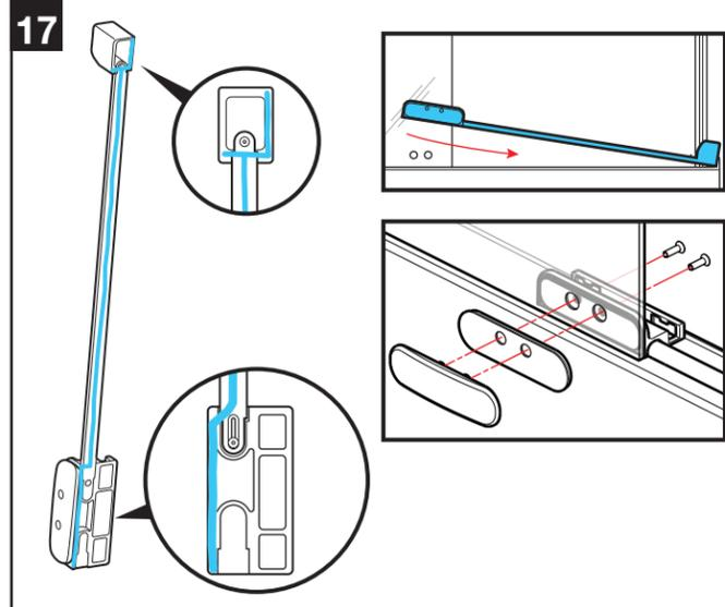
Apply sealant to the threshold bar assembly as shown. Starting with the corner side, lower the assembly into position. Tighten wall mount set screw. Then install foam gasket and door guide plate. Tighten screws. Wipe off the excess sealant that squeezes out.
