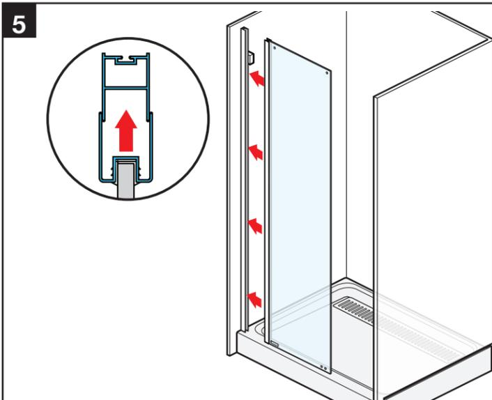
TIP: The joint between the glass panel and wall jamb will accommodate walls that are not perfectly plumb.
