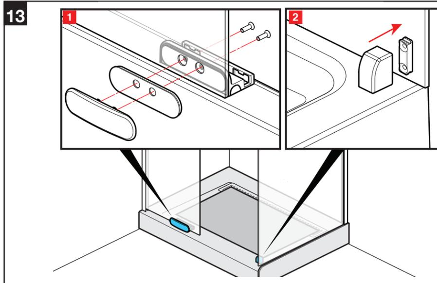
Dry fit the door guide and lower wall mount. Do not completely tighten screws.
