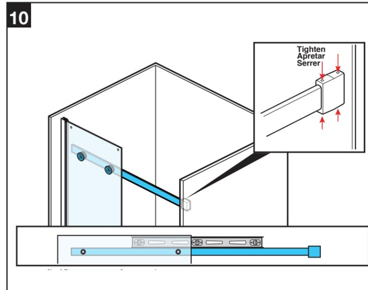
When track is level tighten all screws.
