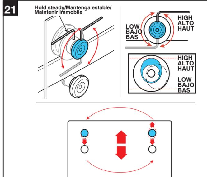
Adjust rollers up or down so door aligns with wall or glass.
