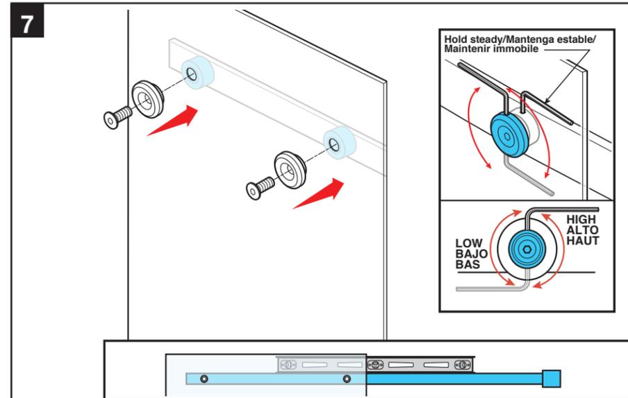
Attach the track to the front glass panel. Adjust mounts up or down to level the track.
