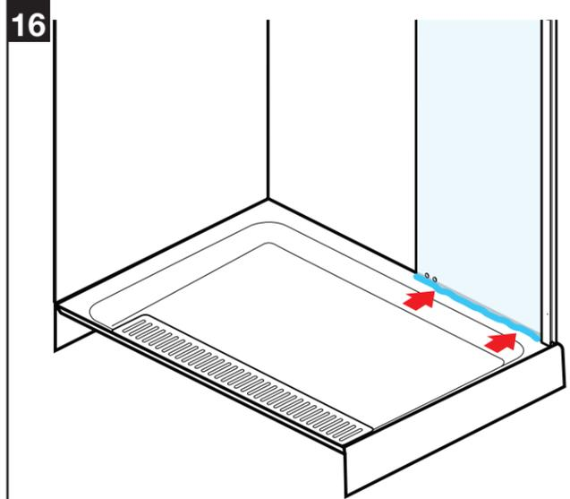
Apply sealant to the inside bottom of the glass panel.
