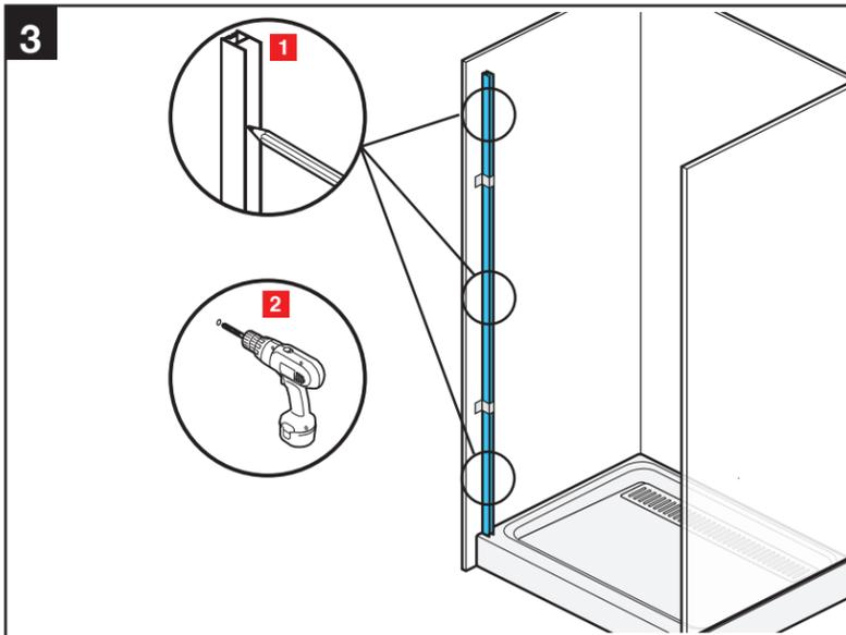
Drill all 3 holes through wall material using a 3/16" drill bit (for tile walls, use a glass and tile bit). Next drill into studs: 7/64" bit for the wall jamb holes.
