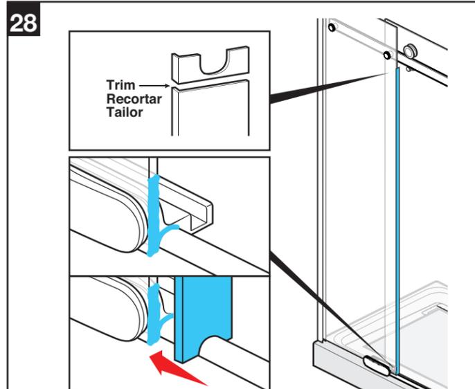
Dry fit gasket and trim the top. Apply sealant to the guide block and install gasket. Clean off excess sealant. Notice: The gasket should contact the base.
