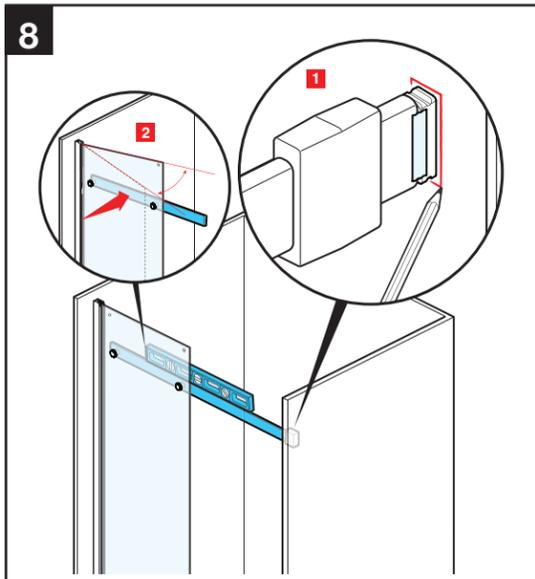
Use tape to position the wall bracket [C] so that it is flush with end of the track. Mark location of bracket on the wall. Carefully angle the glass panel and track inward.
