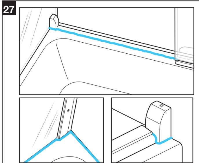
Apply sealant where the wall jambs meet the walls and base. Apply sealant to threshold bar and wall mount.
