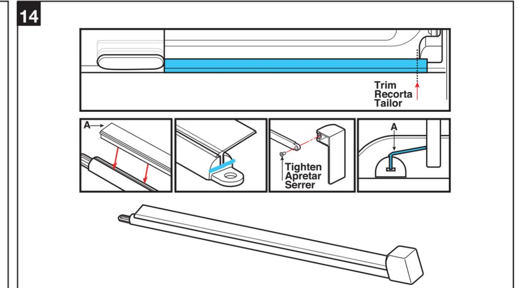
Place the threshold gasket between the door guide and lower wall mount. Trim the gasket to fit. Slide the gasket into the threshold bar. Apply a bead of sealant as shown. Install the lower wall mount.
