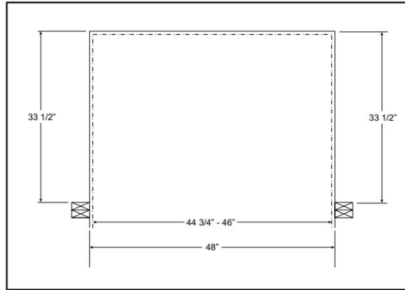
Studs must be in this location on each side for door installation. Other stud locations are not critical.
