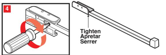
Apply and bead of sealant to the door guide as shown. Install plug [F] and threshold bar into door guide. Slide door guide up against the gasket and tighten the screw.
