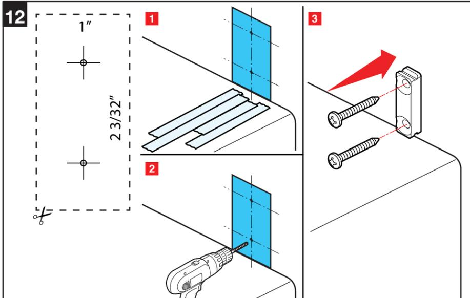
Place masking tape on the base for protection from the drill. Drill holes through wall material using a 3/16" drill bit (for tile walls, use a glass and tile bit). Then use a 9/64" drill bit to drill holes into studs. Install wall bracket. NOTICE: Screws must go into studs.
