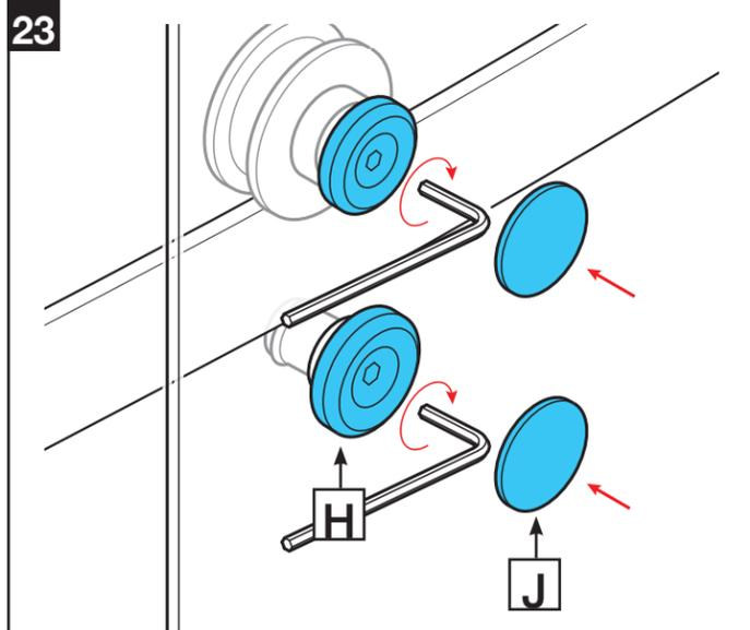
After all adjustments have been made, tighten the rollers and retainers [H]. Install caps [J].
