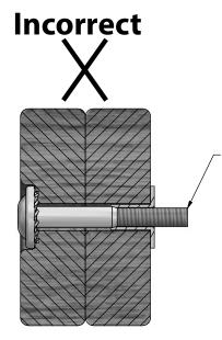
If you see exposed threads and your bolt protrudes beyond the T-Nut you may have over tightened the bolt or used incorrect hardware. If you've overtightened, remove the bolt and add washers to eliminate the protrusion.
