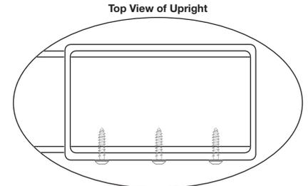
Make sure the rails are in far enough for the screws to make connection to the rail (3-3/8" approximately) inside the upright
