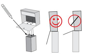
**2** Using a  $\frac{1}{4''}$  drill bit, drill four pilot holes in the marked positions approximately  $1^{1/2^{"}}$  deep into the wood. Attach the Metro to the post using four  $1^{1/2''}$ lag screws. A 1/2'' drive socket or a 1/2'' wrench may be used.
