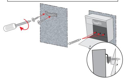
**3** Using a masonry style drill bit(not provided), drill the bottom three pilot holes approximately 2" deep into the wall material. Now hang the Metro from the mounting bracket and secure to bottom using the three 2<sup>1</sup>/4" screws provided. Be sure to put some weather resistant caulk into the holes. If your wall is a thick brick, stucco or concrete you may need masonry screws or anchors for attachment. Consult a contractor if necessary.
