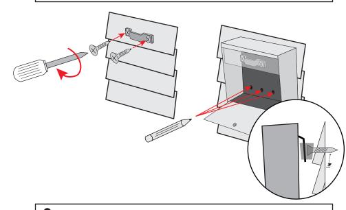
**3** Using a <sup>1</sup>/8″ drill bit, drill the bottom three pilot holes approximately 2" deep into the wall material. Now hangy our Metro from the the mounting bracket. If there is a large gap between the Metro and the wall insert a bushing on the screw. Insert some water resistant caulk into the hole and secure to bottom using the remaining three  $2^{1/4}$  screws provided.
