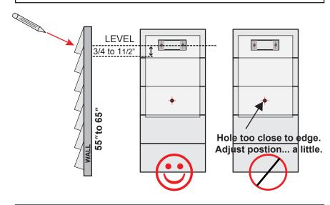
$\mathbf{2}$  Using a <sup>1</sup>/8" drill bit, drill the top two pilot holes approximately 2" deep into the the wall material. Attach the mounting bracket using the two  $2^{1/4''}$  screws provided. Be sure to put some water resistant caulk into the holes. Now hang the Metro from the brackets shown and mark the bottom three holes with a pencil.
