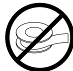
Pipe tape is not recommended.
