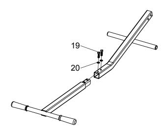
Attach handle bottom to angle frame using bolt, washer, split lock washer, and nut. Insert ring grip pin as shown.
