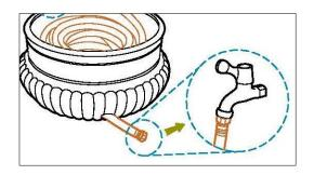
1. Insert the female end of the garden hose through the hole at the bottom inside the hose pot.
